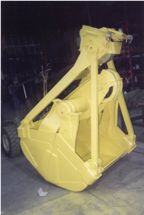
One and one half cubic yard, lever arm clamshell bucket
