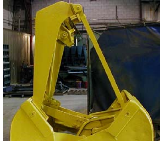
One cubic yard, single line clamshell bucket
