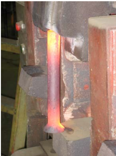
#4 Hook plates are riveted together. Rivets are placed in an electric heater until red hot.
