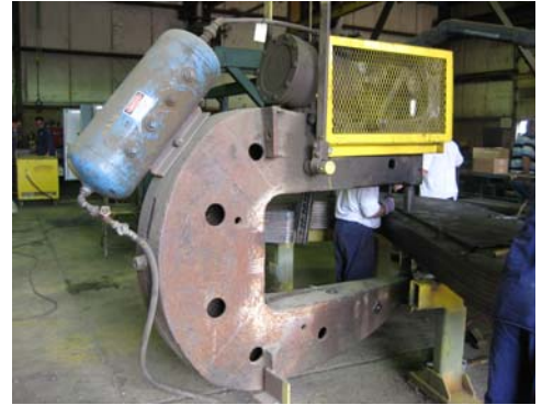
#3 Plate laminations are riveted together using a special air-powered riveting machine.
