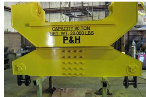
An 80-ton capacity reeved in power rotating ladle beam with fabricated chase blocks and ladle hooks with bronze palm bushings and hardened steel eye bushings.
