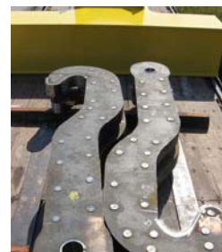
An 80-ton capacity reeved in power rotating ladle beam with fabricated chase blocks and ladle hooks with bronze palm bushings and hardened steel eye bushings.
