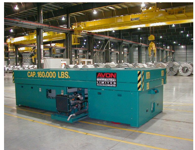
Propane powered transfer car can also be used for handling dies and molds.
